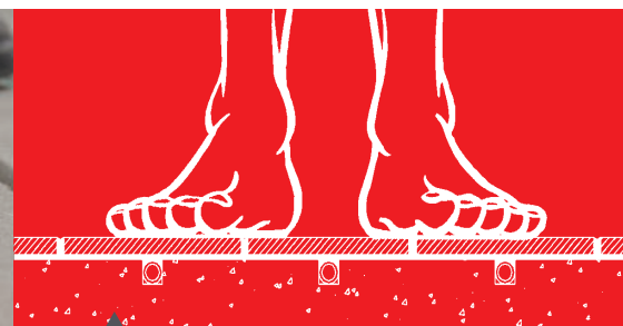
Heating pipes are installed directly under the surface of the floor, for quick heating and precision room temperature control.
